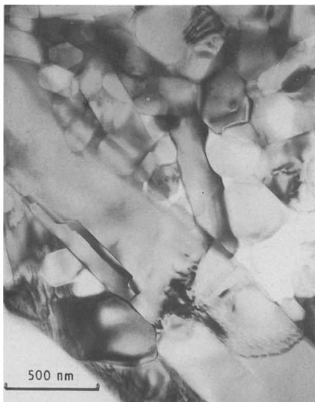
Figure 2 Transmission electron micrograph of an as-sintered \text{Si}_3\text{N}_4 sample.
