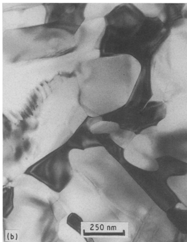
Figure 3 Transmission electron micrographs of a crept sample: (a) microcrystallization, (b) bi-phased microstructure; t = 218 h; T = 1473\text{--}1613 K; \sigma = 200 MPa.
